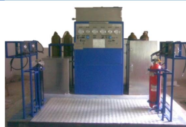
Helium Charging System
