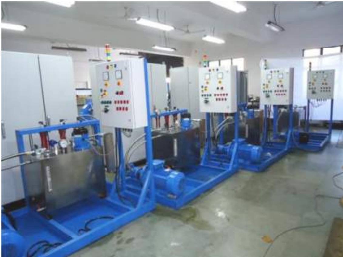
Hydraulic Power Packs designed for AVIATION applications. All pipelines/fittings are SS 304
