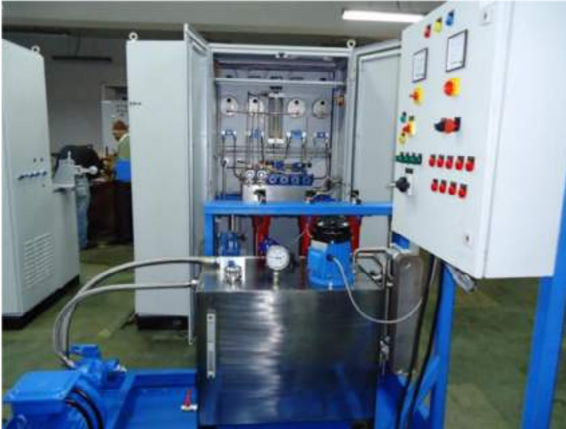
Hydraulic Power Packs designed for AVIATION applications. All pipelines/fittings are SS 304
