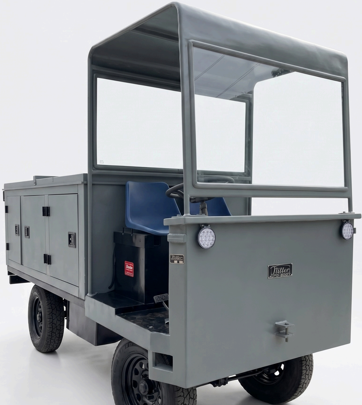
UGSSN2 tow vehicle — self-propelled utility base with equipment cabinets, canopy, and LED work lighting
