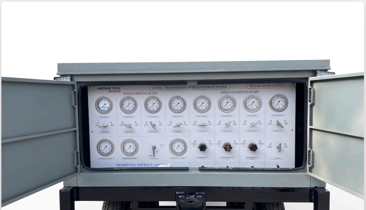
Storage & Boosting / Supply & Distribution panel — open configuration showing full instrumentation array (M/C No. A2700-1/2024)
